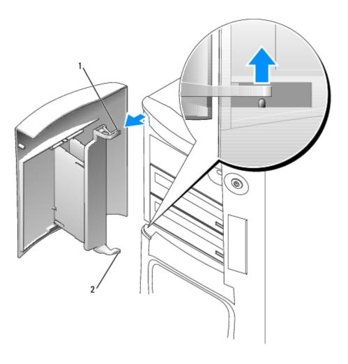
3. Lift the bottom bracket hinge away from the computer.
