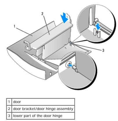
3. Attach the drive door to the computer, starting with the bottom bracket hinge.
