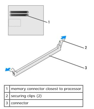
4. Align the notch on the bottom of the module with the crossbar in the connector.
