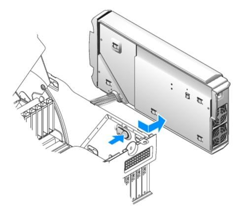
**NOTICE:** To avoid damaging the cables when you reinstall the power supply, replace the cables as shown below.
