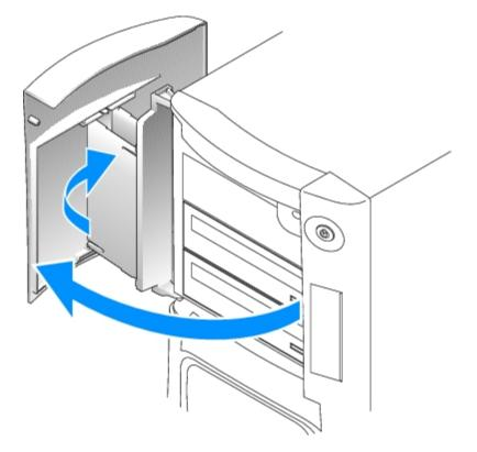
2. Unsnap the top bracket hinge and pull the top of the drive door outward, away from the computer.
