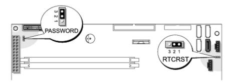
2. Locate the 3-pin password jumper (PASSWORD) on the <u>system board</u>, and attach the jumper plug to pins 2 and 3 to clear the password.
